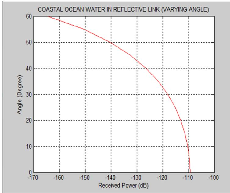
Fig 11: Reflective link scenario for coastal ocean.
