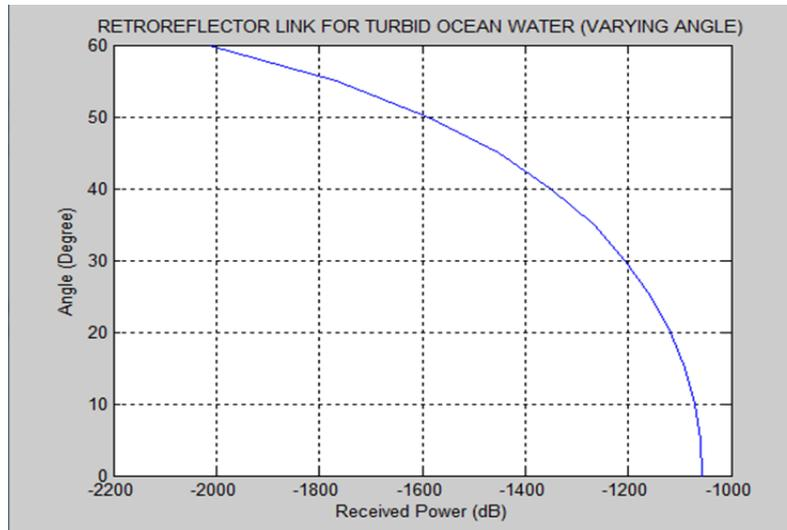
Fig 9: Retro reflective link scenario for turbid ocean (varying angle)
