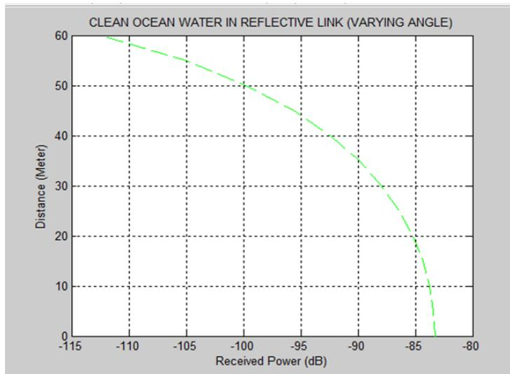
Fig 10: Reflective link scenario for clean ocean
