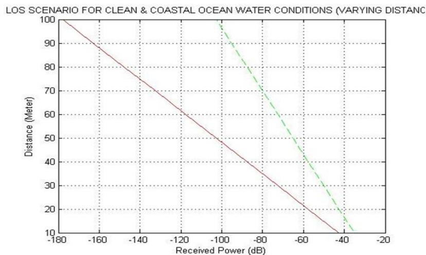
**Fig 1:** LOS scenario for clean (green) and coastal ocean (red) water conditions (for varying distance)
