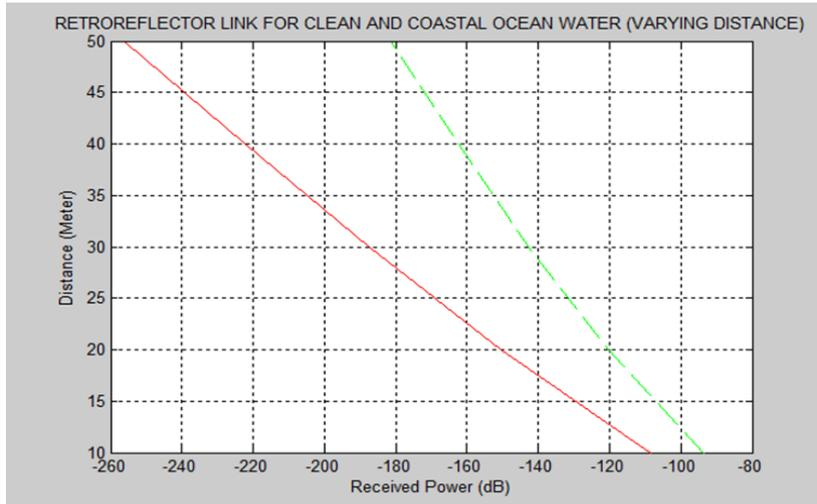
Fig 5: Retro reflective link scenario for clean (green) and coastal ocean (red) (varying distance)
