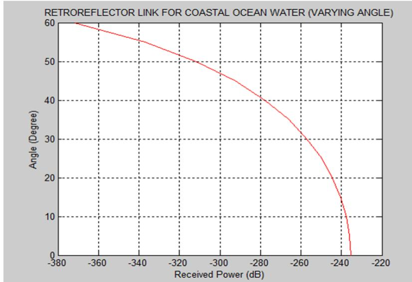
Fig 8: Retro reflective link scenario for coastal ocean (varying angle)
