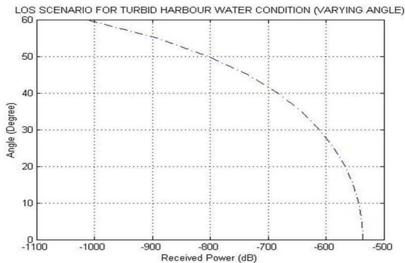
Fig 4: LOS scenario for turbid harbor water condition (varying angle)
