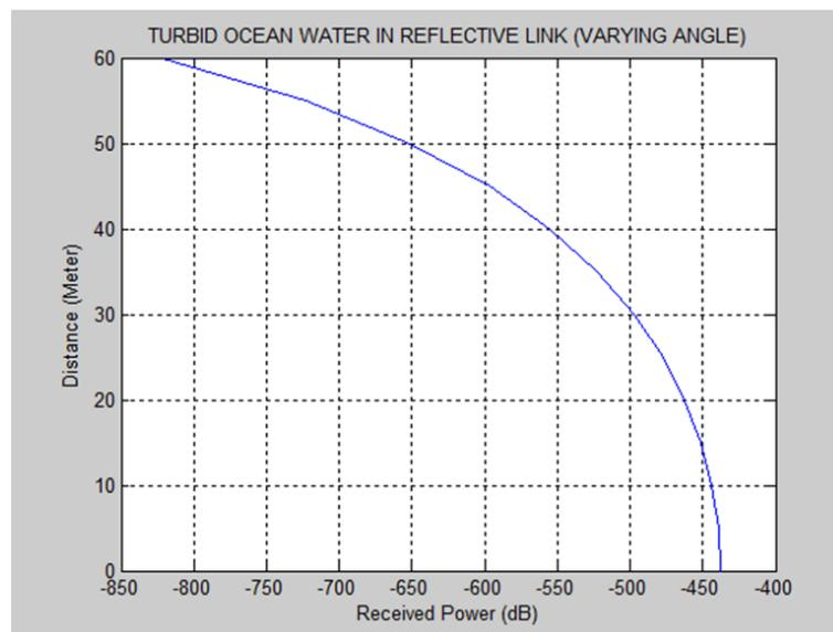
Fig 12: Reflective link scenario for turbid ocean
