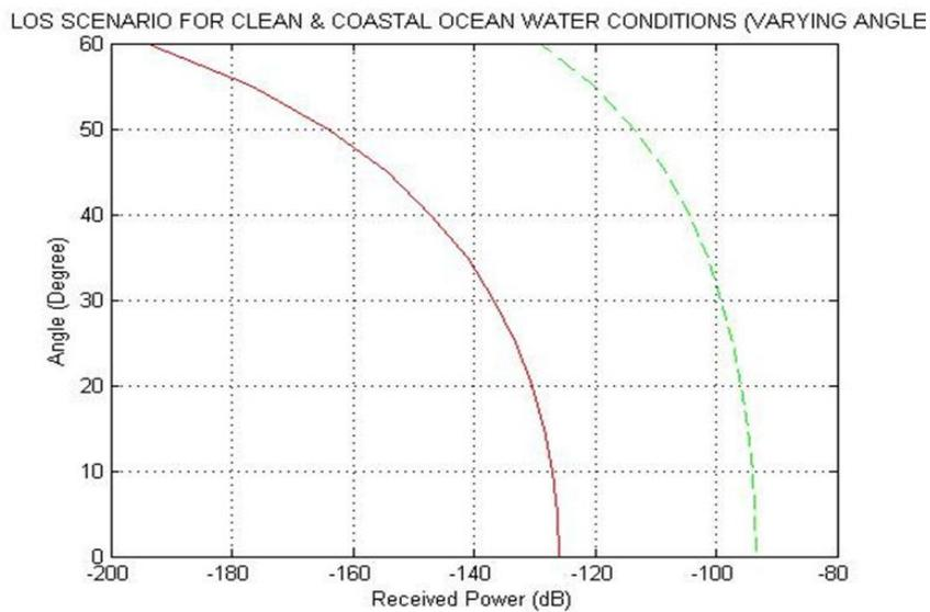
Fig 3: LOS scenario for clean (green) and coastal (red) ocean water condition (varying angle)
